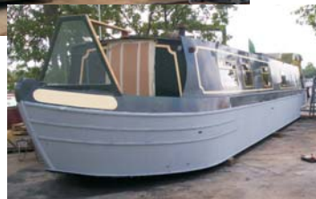
Steel Boat Blasting & Zinga Cold Galvanising
