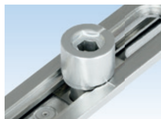
Duplex locking cam with adjustable gasket pressure ( \pm 1 mm). Adjustment with either 4 or 6 mm Allen key
