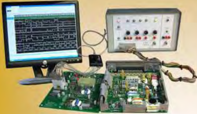
ECU Test Jig
