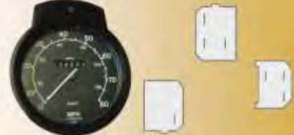
V21C VDO S/ex £95.00 Curved Top VDO Type Analogue Odometer, 3 Plugs 1/4" spades 8 DIL Switches
