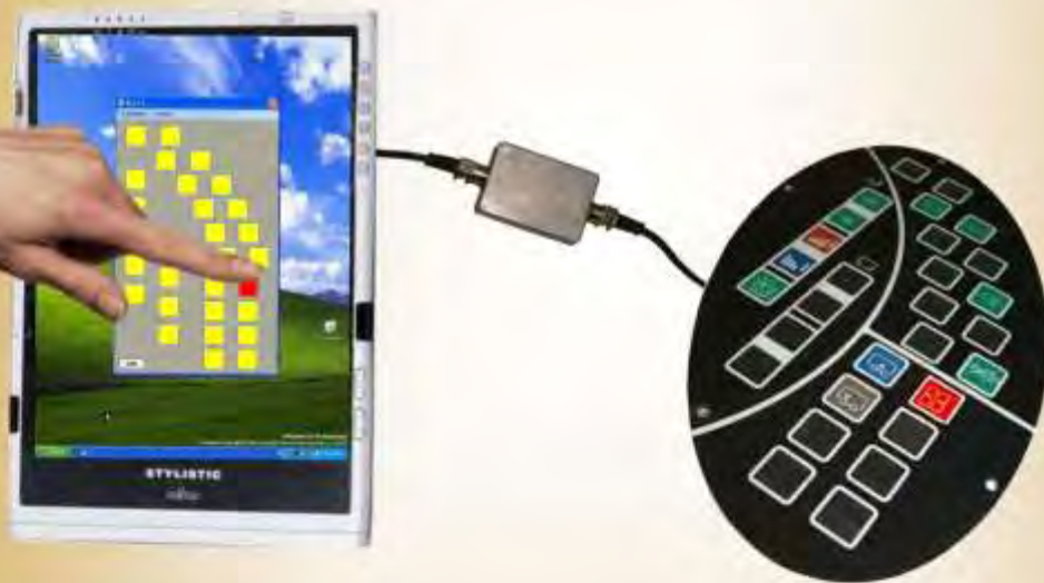
Purpose built Full Test Jig for Volvo B12B dash clusters
