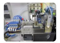
The CPR-ZERO is a fully automatic multi-purpose dual-end processing machine with a small footprint and many possibilities. Servo presses are standard on both sides, twist-flux-solder units can be added to the machine, as well as sealing units. A wire pre-feeding unit is built in to improve wire feeding and processing accuracy, and space saving. With outputs of up to 4 000 wires per hour, and reasonable machine price, the cost per wire can be significantly reduced.
