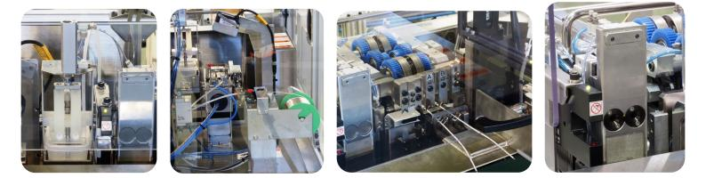
The WDH07 is a 2-wire dual end soldering machine with stripping, twisting, fluxing, and soldering functions. The small footprint of the machine makes it easy to place and operate. With an output of up to 3 600 wire per hour, this is the by far fastest soldering machine in the market. Optional wire handling and pre-feeding systems available.
