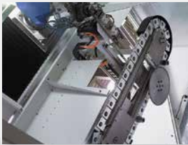
Chain-type magazine with 33 tool places
