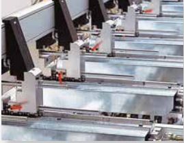
Machine table with 6 steel supporting cross bars
