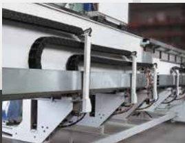
Chip protected supply lines on the back side
