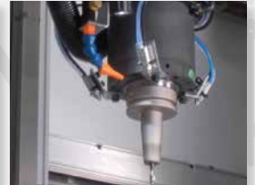
Minimum quantity lubrication, cooling / lubricating nozzle at the working unit
