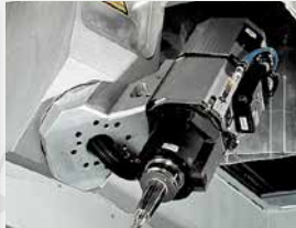
Milling spindle, HSK F63, 10 or 15 kW
