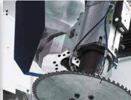
Standard milling unit with gimbal bearing
