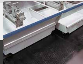
Chip push carts under free-floating cross bars
