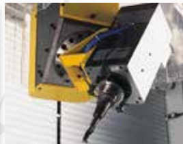
Milling spindle, HSK F63, 26 kW
