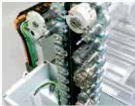
Chain-type magazine with max. 32 tool places
