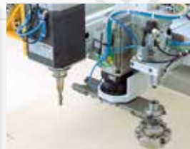
Tool shuttle for rapid tool change
