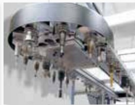
Chain-type magazine with 33 or 51 tool places
