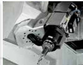
Milling spindle, HSK F63, 10 kW or 15 kW
