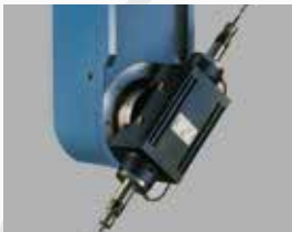
4 kW DFM milling spindle
