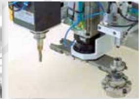
Tool shuttle for rapid tool change
