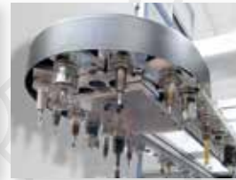
Chain-type magazine with 33 or 51 tool places
