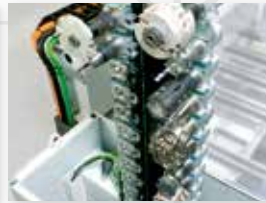
Chain-type magazine with 16 or 32 tool places
