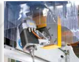
NC-adjustable chip collecting system
