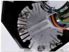
Drum-type magazine with 10 tool places
