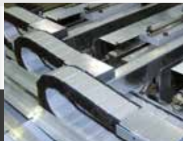
Cable drag chains, closed version
