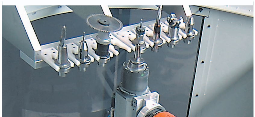
Tool magazine: Linear tool magazine, 8 tool places, C:C 150 mm
