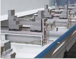
Hydraulic profile clamping units, opening on both sides
