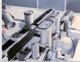
Cross bar table with vacuum pod package
