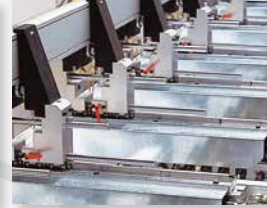
Manual or NC adjustable machine table with steel supporting cross bars
