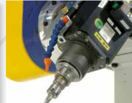
Blow nozzle at the working unit
