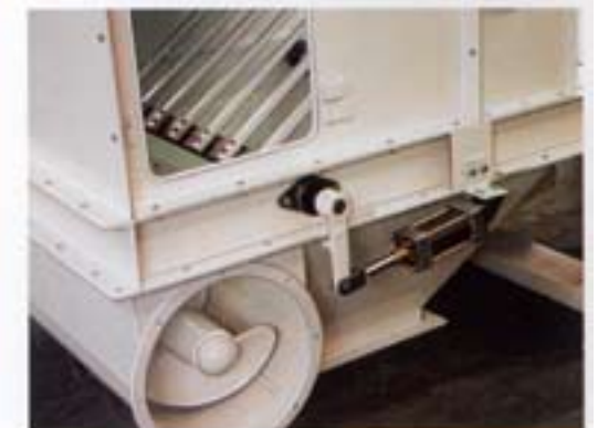
Flattened sacks fall into auger type compactor.
