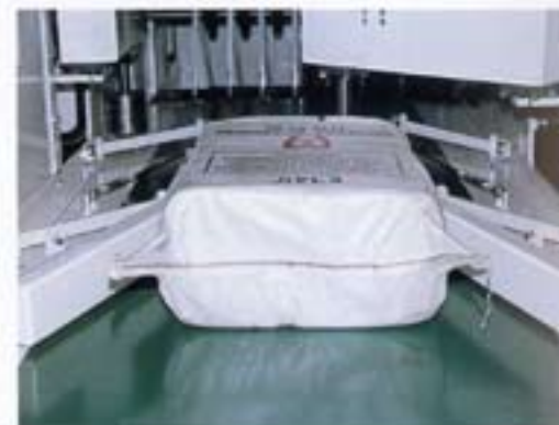
Sack enters machine, detector initiates automatic sequence. Slitters can be seen ahead of the sack in this picture
