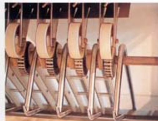
Hook ended levers raise cut sack from belt and separate it from material. Highly efficient recovery is achieved.
