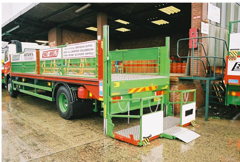
Typical example of a column tail lift with fixed safety handrails
