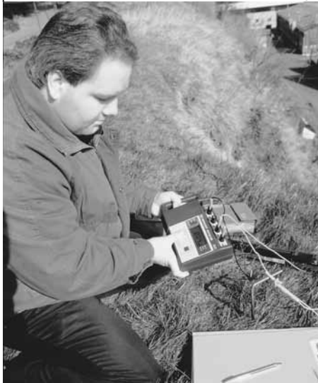
Typical use of a Megger digital ground resistance tester to perform fall-of-potential testing
