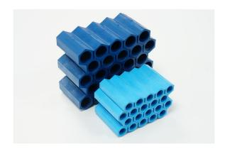
Duct sealing system FiloSeal+HD is a universal solution for sealing larger heavy cables and pipes in ducts, bore holes or transit frames. Upto 2 bar Pressure Resistance 100Kg pulling Force on the cables when sealed 10xd at 45°, with 1 bar pressure bending test
