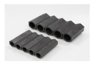
Duct sealing system FiloSeal+HD FIRE is our new highly certified fire, gas and water sealing system for both ducts and transit frames Up to 4 hours fire resistance in transit frames (single side) Up to 4 hours fire resistance in ducts Tested to BS EN1366-3 2009 Upto 2 bar Pressure Resistance 100Kg pulling Force on the cables when sealed 10xd at 45°, with 1 bar pressure bending test
