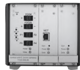
Single-camera rack with video server
