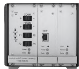
Single-camera rack with video server
