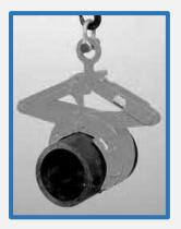
Other <u>steel sections</u> such as tubes, angles, channels, universal beams and railway lines can all be lifted by standard clamps designed for the particular section.
