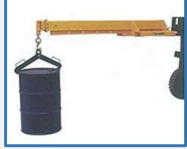
This method of handling is much safer than balancing an unstable load over the forks and provides the ability to rotate and position the load much more safely and precisely. (Continued)
