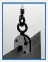
Generally the initial grip of cam types comes from a spring operated by a lever which the user flips over into the locked position after positioning the clamp on the plate.
