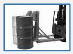
In addition to drum clamps which slide-on to the forks of forklift trucks, there is a wide range of drum lifters for use with an overhead crane or hoist.
