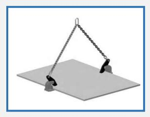
As the name implies, horizontal plate clamps only handle plate laid flat. They are therefore always used in pairs, one either side of the plate, in conjunction with a two leg sling.
