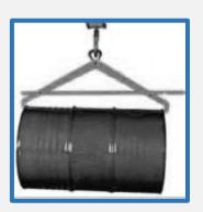
In addition to lifting drums vertically, there a clamps which lift drums in the horizontal position.
