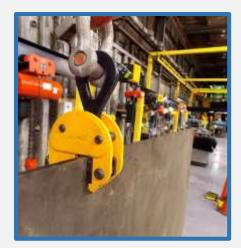
Clamps are the ideal tool for handling loads safely by overhead crane or hoist.
