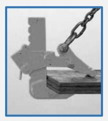
Variations of this type of clamp include designs for handling single plates within a range of thickness, to be adjustable to handle several ranges, or to handle bundles of several plates.
