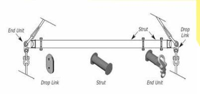
configuration required. Lifting beams and spreaders of these types make it cost effective for one off or limited applications.
