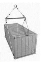
Lifting beams and spreaders are often used when there is limited headroom. Ideally it is best if the attachment points on the load are above its centre of gravity as that will ensure that the load will always hang in a stable position.
