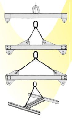
A lifting beam is loaded in bending. Typically a simple lifting beam will have a single lifting eye above the beam which engages with the lifting machine hook and lower lifting eyes at points on the underside of the beam to connect to the load.
