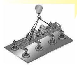
Most lifting beams and spreaders will be designed for specific applications e.g. A lifting beam for use with vacuum pads or lifting magnets to lift long flexible loads which needs support at regular intervals to
