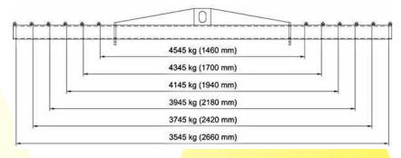
There are two basic approaches to this. Lifting beams can have adjustable lifting points which can be moved along the beam to suit the particular load.
