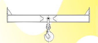
This facilitates tandem lifting. The total lifting capacity can be that of the two cranes less the self-weight of the beam and any allowance for uncertainty in the sharing of the load.
