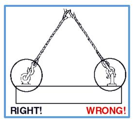
Although a collar eyebolt is designed for angular use it is nevertheless necessary to align the eye to the line of pull. A tolerance of  $\pm 5^{\circ}$  is acceptable but it is a matter of luck whether this will be achieved when first screwed in because the eyebolt manufacturer has no control over the start point of the threaded hole. Therefore it is permissible to shim up to half the screw pitch to achieve the correct orientation.
