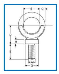
Dynamo Eyebolts - metric coarse thread - For Axial loads only (NOT TO BE USED FOR ANGLED LIFTS)
