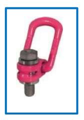
**VLBG Load Ring** will turn 360°, adjustable in pull direction. Load ring foldable, full WLL in any load direction, surface pink powder coated. The max. lengths of the RUD - bolts are adjusted in such a way that if a hex-head-shaped nut (DIN EN ISO 7042) is used, assemblies of material thickness of approximately 8 \*M
