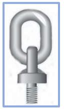
The eye of a collar eyebolt is too small to accept a hook so a shackle is always needed as the first item of any connection. However BS 4278 does offer a third option and that is the eyebolt with link.
