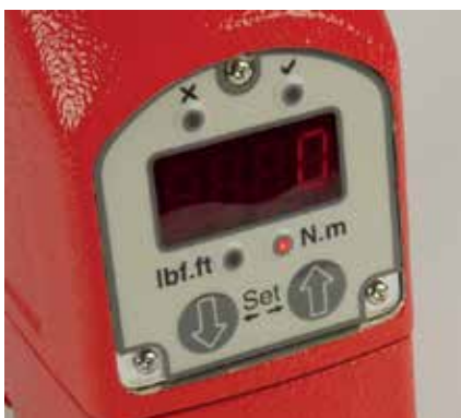
Internal Control (IC) Panel
