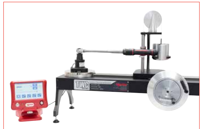
Torque Wrench Calibrator (TWC) manual shown with Counter-Balanced Reaction Post (62272), Flange Mounted Transducer and a T-Box XL™
