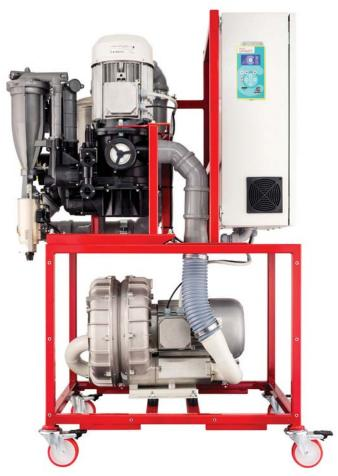
In addition to the features already mentioned, it should also be noted that the centrifugal separator in Maxi Smart replaces both the centralized separator tank and the Turbo Smart (used as drain pump), greatly reducing the size of the plant and greatly simplifying maintenance operations.
