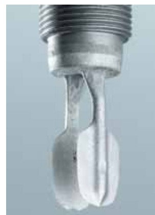
Frequency change due to corrosion (maximum alarm)
