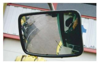
Wide angle mirrors aren't limited to use on trucks only, they are used in different applications to improve safety. The class IV & V approved M430CE can be seen above mounted onto a piece construction equipment. It is being used to help meet a visibility standard.
