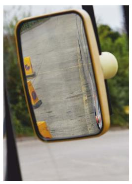
When the Ashtree Cyclesafe twin lens mirror is fitted we have a completely different view. The invisible cyclist is now fully visible, as is the kerb and the door way.
