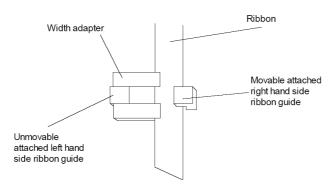
This diagram is based on looking at the open ribbon printer head on. The right hand ribbon guide must be pushed in far enough to just touch the edge of the ribbon and so ensure a straight print.
