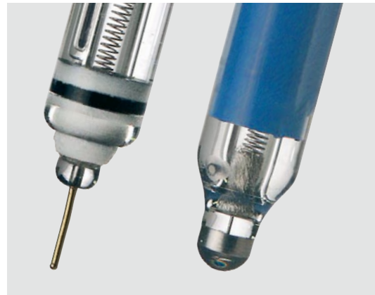
Gold pin or platinum ring as measuring electrode
