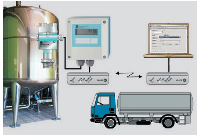
Molasses level measurement in customer specific tanks of a supplier. The Minilog B stores the customer usage and informs the supplier of the actual level in the storage tank. The data is collected at a central supply point and are available for the planning of just in time delivery.
