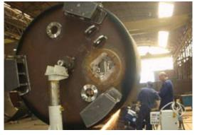
GBC G400 shown mounted on trolley, during typical back grinding operation, circumferential on O.D. of pressure vessel. The trolley allows easy handling and moving of the grinding head.
