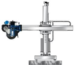
GBC G400 mounted on column welding boom arm, equipped with needle bearing kit for 360° rotation. This layout allows for back grinding circumferential, longitudinal, outside and inside on large diameter vessels.
