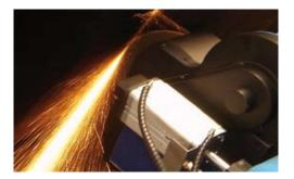
G 400 Grinder head feeding system is pneumatic with compensation which retracts the feeding piston when it senses meeting ovality.
