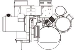
Grinding head can turn of 90° for dedicated set up when performing longitudinal back gouging (mounted on column welding boom arm only).
