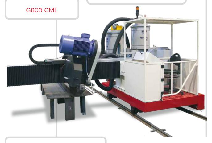
The machine is completely electronic, equipped with brushless motors, and can be remotely operated for the main functions, while the LCD monitor connected to an HD video camera enables the operator to have a constant visibility on the machine work.
