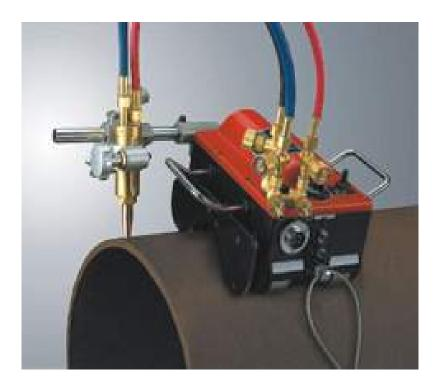
With two sets of internal magnetic rollers the GBC MAGCUT can be used for parallel, vertical and downhill cutting. The robust aluminium body construction makes this unit both durable and easy to operate.
