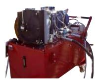
Hydraulic power pack oil tank 250 L, with remote control and inter-cooler for extremely heavy duty working session & environmental
