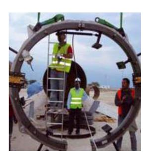
The Hypercutter is a split frame design for ease of set up and operation along pipelines.
