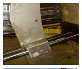
The unit is also equipped with two copier toolboxes with the spring loaded pipe OD tracking system, minimizing the bevel offset on out of round pipe.
