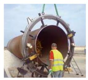
A hydraulic cold cutting and beveling machine for the heaviest of applications, suitable for factory or on-site work.
