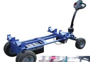
Originally designed to create a bespoke transport solution for a pipework installation project, this motorised trolley is ideal for securely moving heavy pipes and tubes around congested sites.
