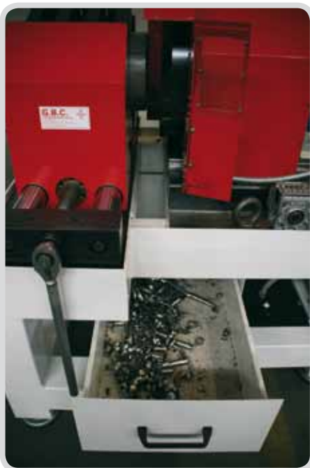
Detail of the chips collecting tray
