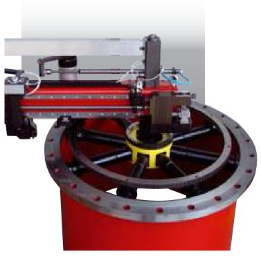
Our multi position motor always creates the minimum distance between the cutting point and power transmission. Thus eliminating chatter and achieving higher cutting speeds.
