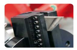
The unit is equipped with easily interchangeable tools for any angle of bevel which come in various hardness scales in relation to the material typology:
