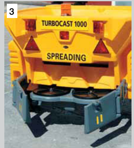
Repeat the procedure for the second side deflector to complete the conversion.
