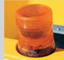
Amber flashing light
