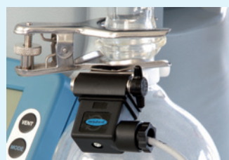
Liquid level sensor for VACUUBRAND catchpot 500 ml
