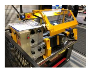
a fully-compliant Harrison M300 lathe fitted with the new TW RAD interlocked guard with gas strut assisted lift and lock (left)
