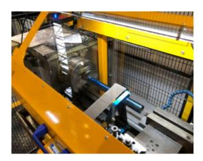
operator's view of the Spider 50 sanding/polishing tool working through the new TW RAD interlocked chuck guard (left)
