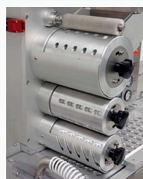
Rectification Station Feed, Rectifier & Transfer Drums
