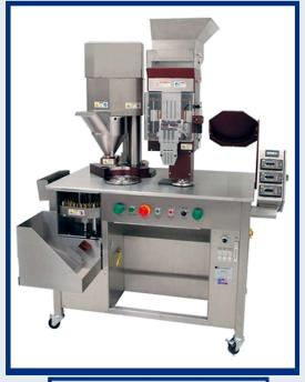
The digital Micro-Drive controllers provide precise adjustment and repeatability for setting the RPM of the Auger and the rotational speeds for the Fill Table and Rectifier Table.
