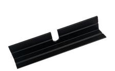
Extruded aluminium mounting brackets allows for mounting of Series 1 - 4 & KFL Range 1 - 4 Enclosures to walls, panels, bulkheads and any other surface. The mounting brackets are secured into place once the end plates are screwed down on to the enclosure.
