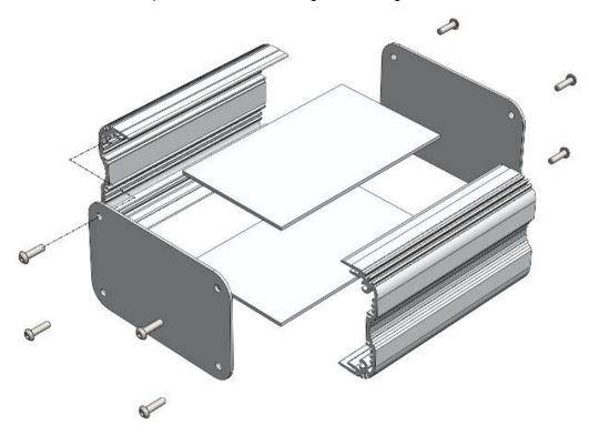
**Length Tolerance of extrusion:** Nominal length +/-0.3mm e.g. U66S160 is not shorter than 159.7mm and not longer than 160.3mm.
