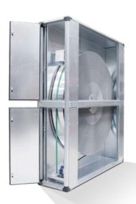
When outdoor air is warmer than the exhaust airflow there is a need for cooling. The hygroscopic rotor then reduces temperature of the incoming air. Simultaneously it transfers moisture from the inbound to the outbound air flows (in cases where absolute humidity is higher outdoors).
