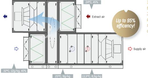
The RegAsorp dehumidifies the supply air by transfering 3g/kg directly to the exhaust air. This enables massive savings on chillers and cooling coils.
