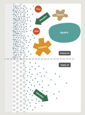
Example of moisture recovery. The picture illustrates how the RegAsorp through adsorption selectively recovers moisture from the exhaust air, and transfers it back to the building via the supply air through desorption.
