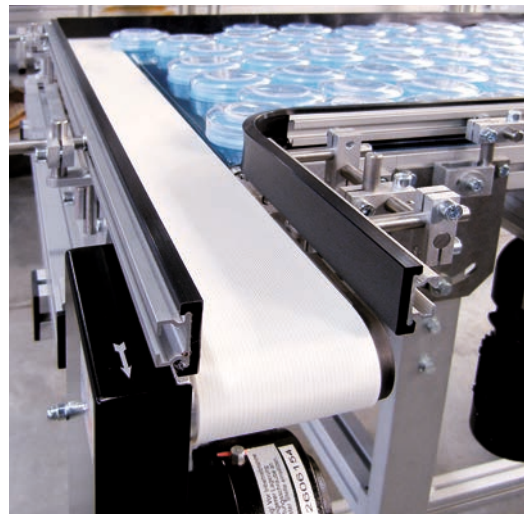
GUF-P 2000 as transverse conveyor and singulator following a cooling section
