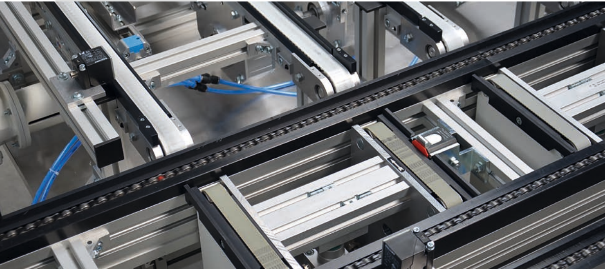
Versamove plus: Transfer of pallets from main line onto two parallel spur lanes
