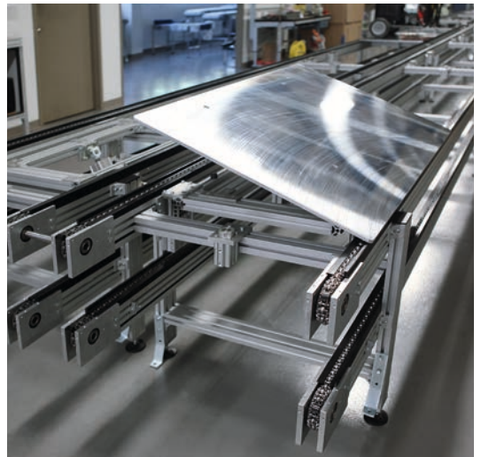
Versamove plus: Two transport levels, accumulating roller conveyor
