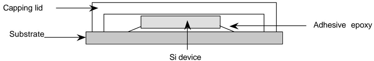
Figure 1: Illustration of the package construction which was cut using the Model 850 Wire Saw. The main areas of interest are where the die interfaces with the various package materials. These areas are where cracking and delamination normally occur during the cutting process.
