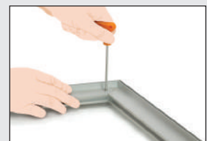
Corners assemble easily with an Allen key [supplied with kit].
