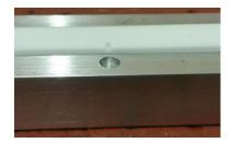
2. Place thermocouple through hole in jaw:
