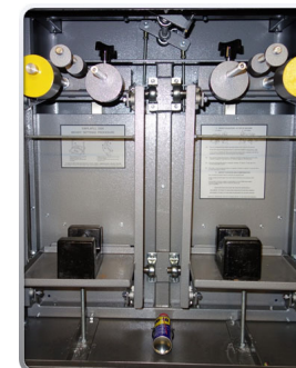
Internal mechanical weighing mechanism of the S2000GR.
